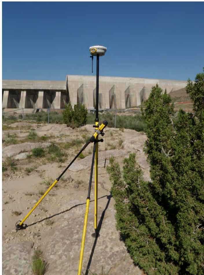
Figure 9 - Reclamation monument "Blake" in solid rock, looking northwest.
