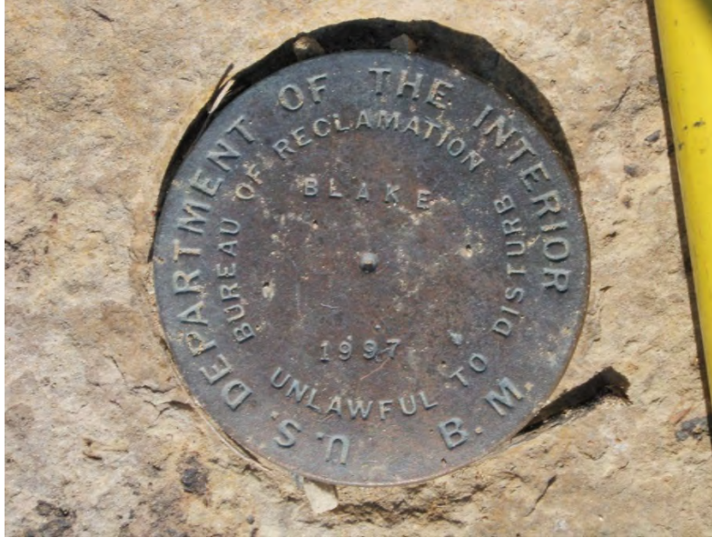
Figure 8 - Reclamation brass monument "Blake" located on right bank downstream of dam.
