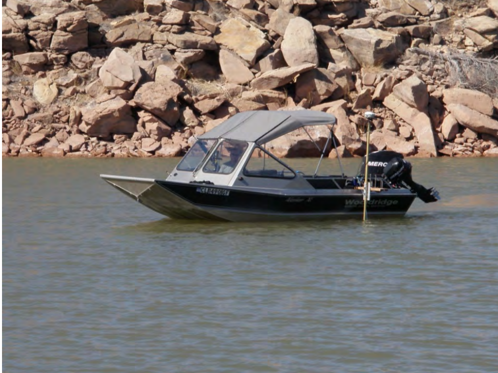
Figure 12 - Survey vessel for reservoir mapping with mounted single beam transducer on side (Lake Sumner-New Mexico, March 2013).
